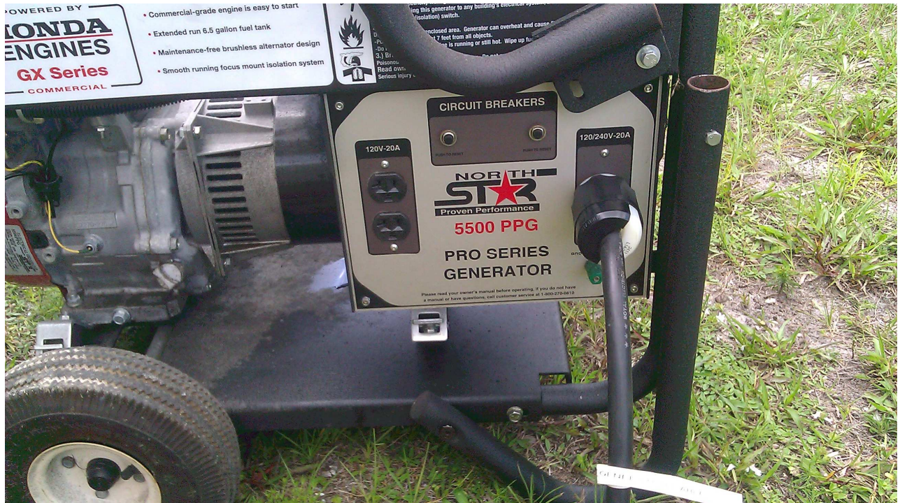
Figure 6. Power Cord Connection to Generator.
