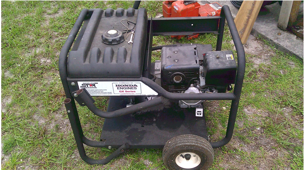
Figure 4. Emergency Generator Removed from Shelter..
