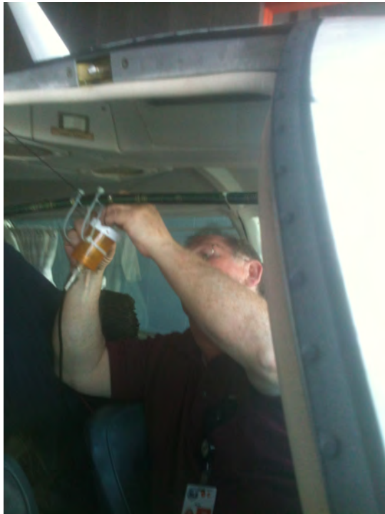
[AD4ES tightening the Balun on Antenna 2]
